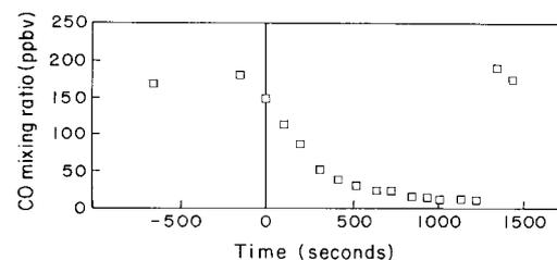
Fig. 1. Change of CO mixing ratios in the flux chamber during a typical experiment. At time=0 the chamber was closed and re-opened at ~1300 s. Mixing ratios before and after the experiment reflect ambient CO levels.
